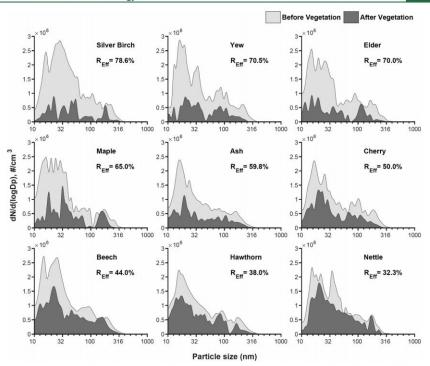
Figure 1. Mean particle number distribution pre- and postexposure (35 min) of each vegetation species to the diesel exhaust ("Before Vegetation" = upwind of vegetation block); "After Vegetation" = downwind of vegetation block).  $R_{Eff}$  (%) indicates the removal efficiency of UFPs by each species.
