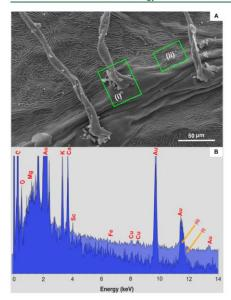
Figure 5. (A) Scanning electron micrograph of the adaxial surface of the pre-exposure silver birch leaf and (B) EDAX spectra for the leaf-deposited PM in subareas (i) and (ii) of image A (note that the sample was gold-coated).
