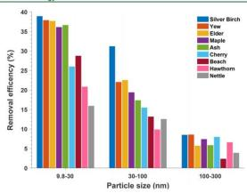
Figure 2. UFP removal efficiency of different plant species for different particle size bins.
